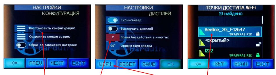
If your receiver does not work properly, you can restore the settings previously saved to the file using the appropriate item in the list, or by pressing the encoder button when the receiver is turned on to reset to factory settings.
