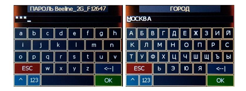
This on-screen keyboard appears when it is necessary to enter characters and data on the receiver pages, the password of the Wi-Fi access point, the firmware activation key, editing the names of memory stations, cities... and much more. Use the "^" and "123" buttons to activate uppercase/lowercase/numeric/special characters. OK to confirm. ESC to cancel.
