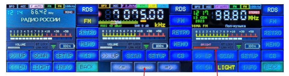
The appearance of the screen with the FM button activated. You can switch the FM band stations stored in the memory bank for the current city with the encoder. The on-screen encoder is activated by dragging from the bottom up at the bottom of the screen. To close, swipe down from the center of the screen. Available in all modes. The appearance of the screen with the LIGHT button activated and the display brightness indication adjustable by the encoder.
