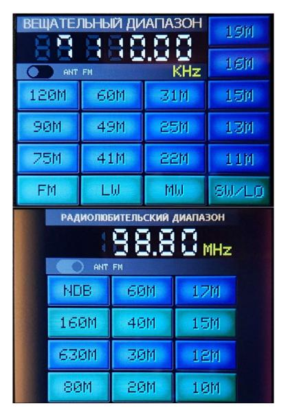
A screen for selecting the broadcast range, with an indication at the top of the currently used frequency.
