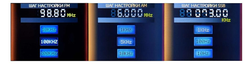
Setup step selection screens for FM - AM - SSB bands.
